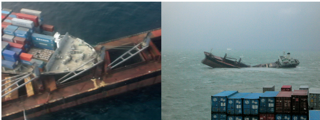
This collision led to the total loss of the bulker. The container vessel had a speed of over 20 knots at the time of the collision.
