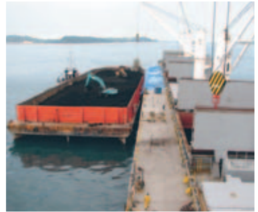
Lightering operation in progress.
